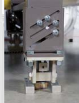
Conveyor Leg Load Cell
